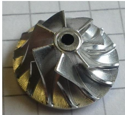
Figure 9: Impeller of compressor C with a 13mm diameter.
