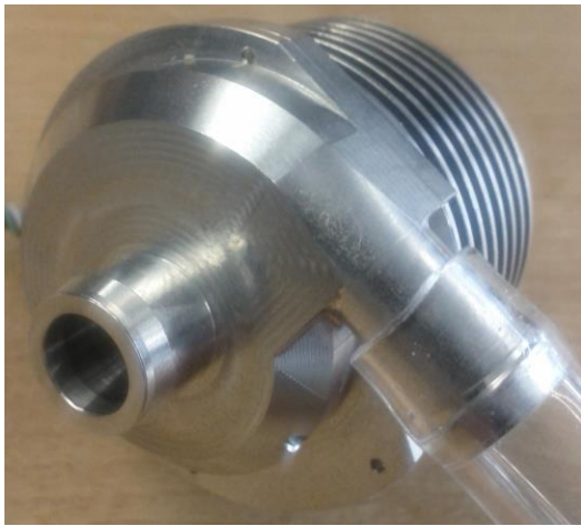
Figure 8: Compressor C prototype. Length 50 mm, motor casing diameter 20 mm, compressor casing diameter 48 mm.
