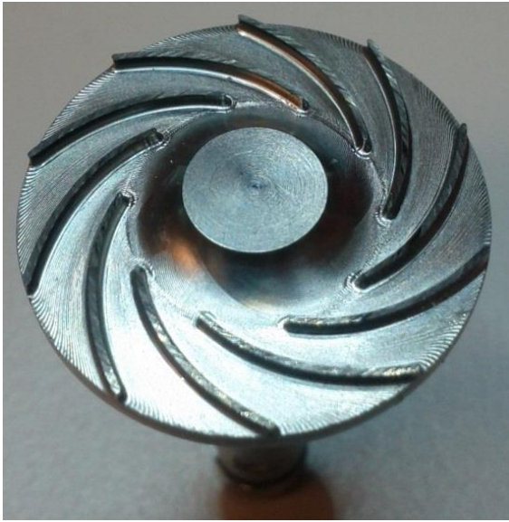
Figure 6: Impeller of compressor B, diameter: 21 mm, rotor length: 36 mm
