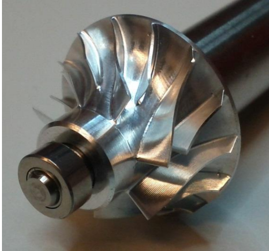
Figure 10: Assembled rotor D including impeller and high-speed ball bearings. Length 69 mm, impeller diameter 21 mm.
